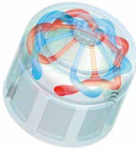
manufacturing specialists analyzed CurTec's difficulties and proposed re-engineering the sprue bushing and sprue bush cooling systems. The team came up with a design of a larger injection opening and 3D printing of the re-engineered sprue bushing with conformal cooling. This became the perfect solution to solve the customer's problems.
