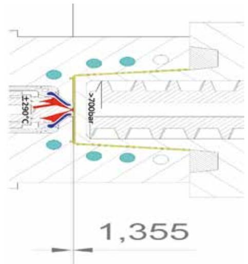
Fig. 2. Sprue bushing in front of the cavity.
